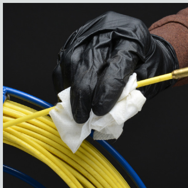
Revitalize fiberglass rodders
