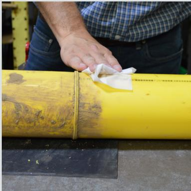
Removing dirt with the EFW-1
