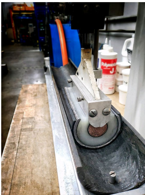
Conduit and cable on the friction table
