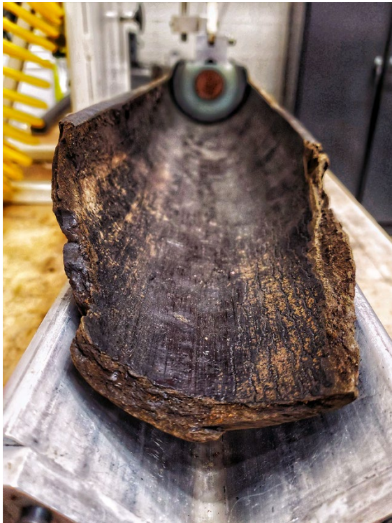
Early example of fiber conduit on the Polywater friction table
