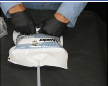
Burst secondary seal
