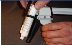
3. Insert cartridge into the wide opening on the black retaining collar.
