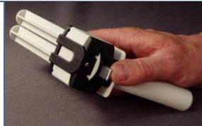
2. While lifting the metal tab, slide piston with ratchet teeth side down, into the slot through the front end. Push the piston all the way through and gently release the metal tab. The metal tab should catch on the ratchet teeth.
