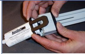
4. Push the collar back and press firmly to snap into place.
