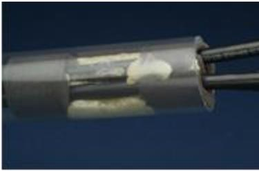
8. Remove burst pack after all material is injected. Sealant may seep between the crevices of the foam dam as it expands. After cure, excess foam may be trimmed and removed.
