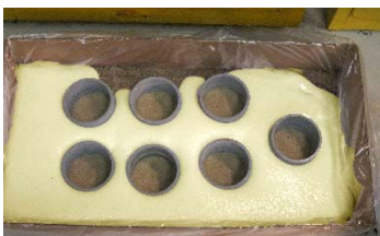
PedFloor flows and expands after 20 minutes
