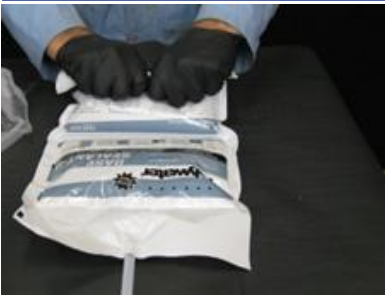
Burst primary seal
