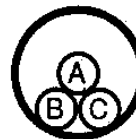
Figure 7. Cable A was pulled on top of in-place cables B or C
