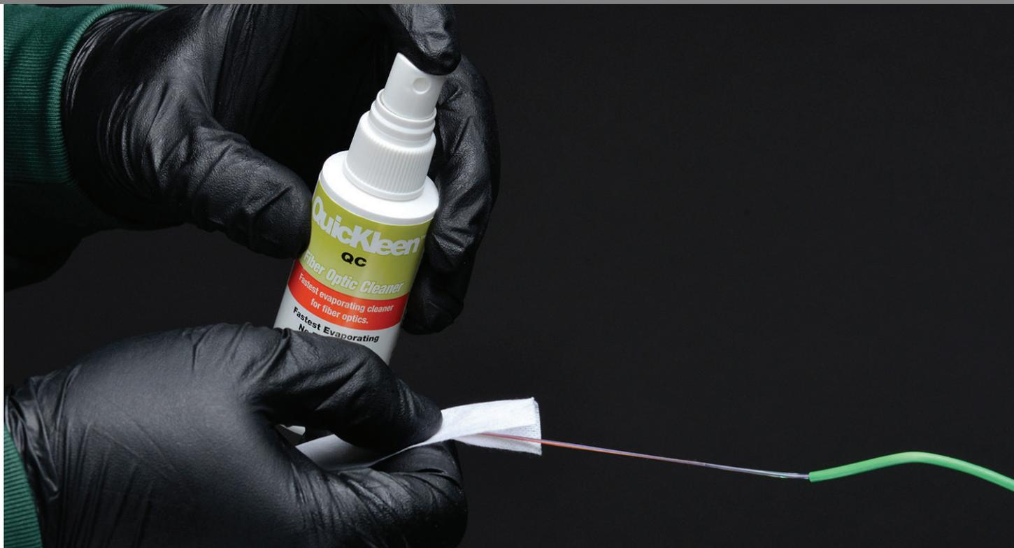
A fast-acting cleaner for ferrules, bulkheads, and fiber endfaces
