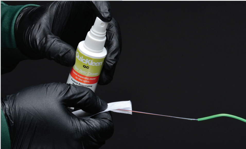
Cleaning fiber with a QC-2LP spray bottle
