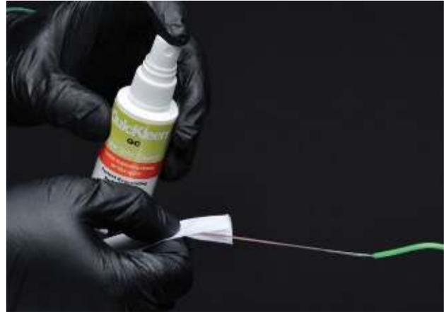
*QuickKleen Fiber Cleaner evaporates quickly without residue.*
