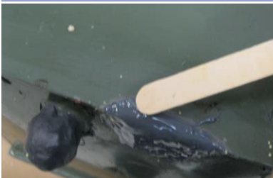
Smooth edges of PowerPatch
