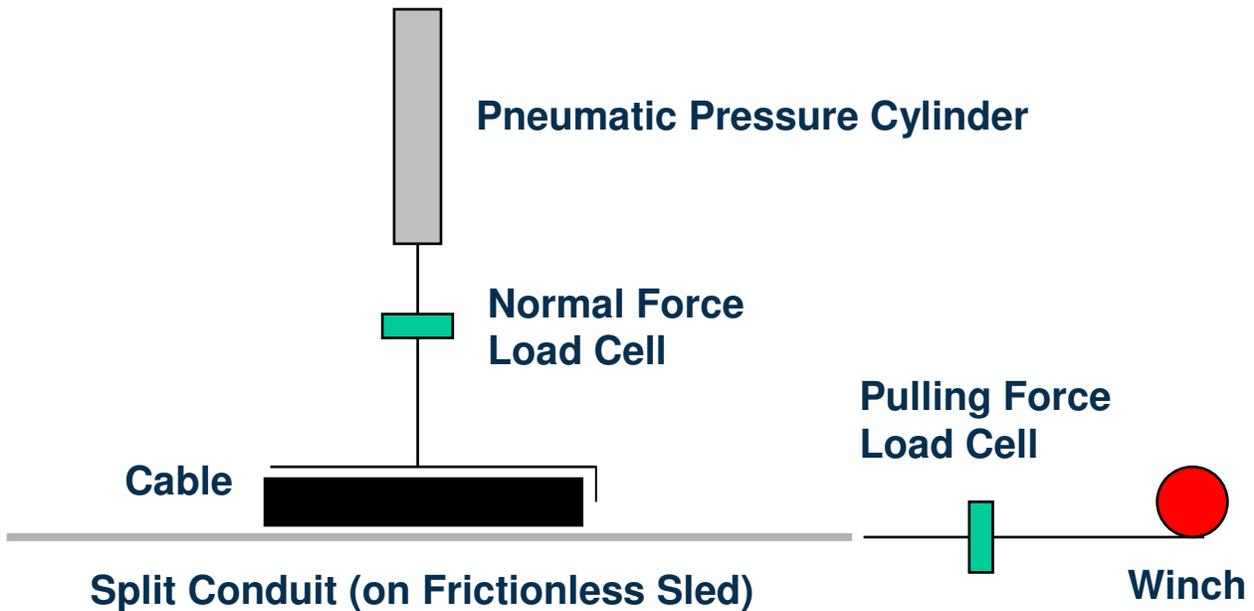
To make a measurement, a section of cable, typically 6 inches (152 mm), is placed on the split conduit. If the test is “lubricated”, the cable and conduit are coated with a thin film of the lubricant. While any type of cable and conduit can be used, the cable must be rigid enough to allow the conduit to slide without the cable bending back on itself.
