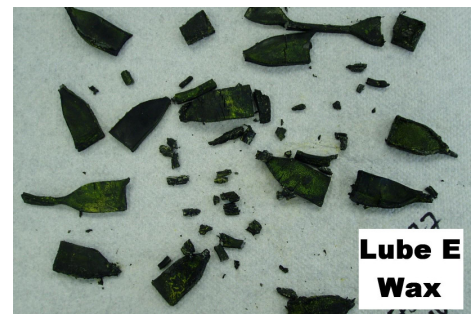
Damaged Jacket Specimens
