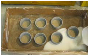
InstaGrout™ is mixed and poured
